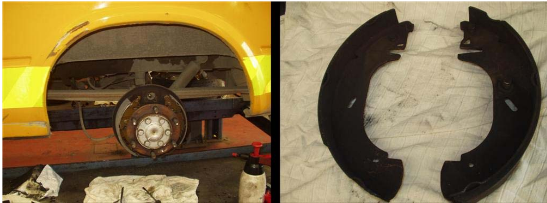
Figure 18.1 Asbestos in brake shoes on a truck
